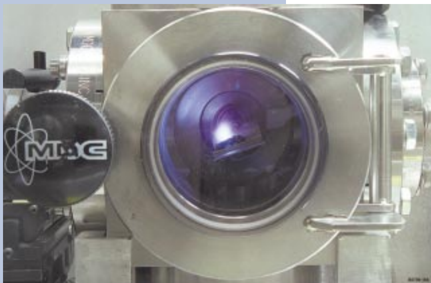
Figure 1. A LIBS plasma plume produced from a lump of electrorefined Pu metal. The laser impinges on the sample vertically from the top, with emission collected horizontally by the 40 mm diameter, f/3 lens at far left. The sample chamber viewport is approx. 2.5" in diameter.
