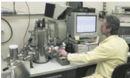
Figure 1. UHV scanning Auger spectroscopy/EELS instrument located in the Chemistry and Metallurgy Research building at Los Alamos. This instrument is used for fundamental actinide surface science research, plutonium physical properties measurements, and analytical surface characterization.
